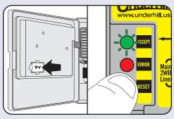
Green ACCEPT light will flash within 8 seconds if module is seated properly. Contact Underhill if green light fails to flash.
