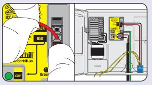
Using module's built-in programmer (Page 13). Be sure zero time is set on all unused stations (up to 48 stations are available in each program A, B, C, and D)
