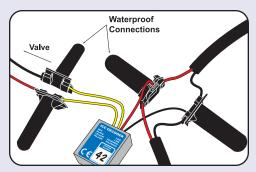
Connect decoders and valves securely. Polarity (+ or -) (red/black) is not important.
