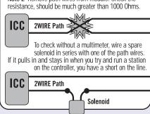
Note 3 Remove decoder. Place onto 2Wire path terminals on module, removing main path wires. Temporarily wire a good solenoid to the decoder under test. Try and operate it from the controller.
