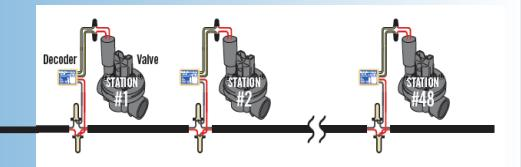
**2Wire Backbone to Typical AC Solenoids**
