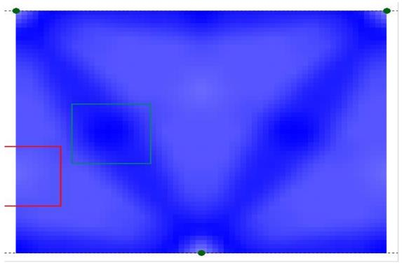
Figure 2. Denso-gram of the Sprinkler and Replacement Nozzle Application Uniformity
